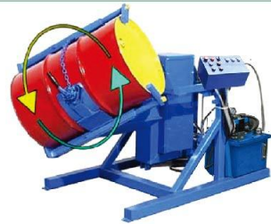
DB360-YD350 电动液压升降单臂滚筒机 Electric hydraulic lifting single-arm roller
