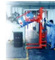
TYG-EX称重型翻转倒料车 Pneumatic explosion-proof rotary batch turning truck
