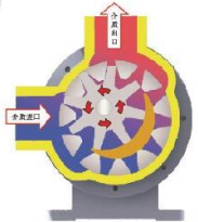
CB 型内啮合齿轮泵工作原理图 CB type internal meshing gear pump working principle
