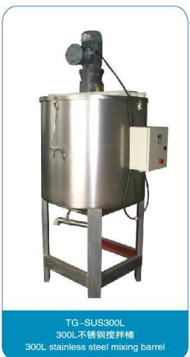
TG-SUS300L 300L 不锈钢搅拌桶 300L stainless steel mixing barrel
