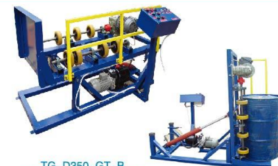
TG-D350-GT-B 自动定时混合机 (附防护栏) Autotimer mixer (Attached protective guard)
